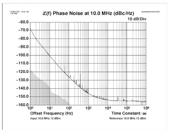
Figure 3.14 Typical GPSTCXO Phase Noise
