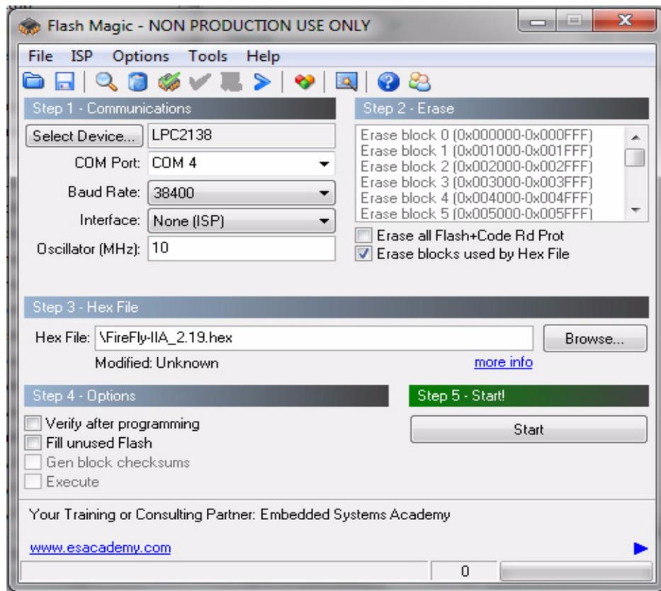
B) Press the “Select Device” button and the window shown in [Figure 4.5](#) will appear:
