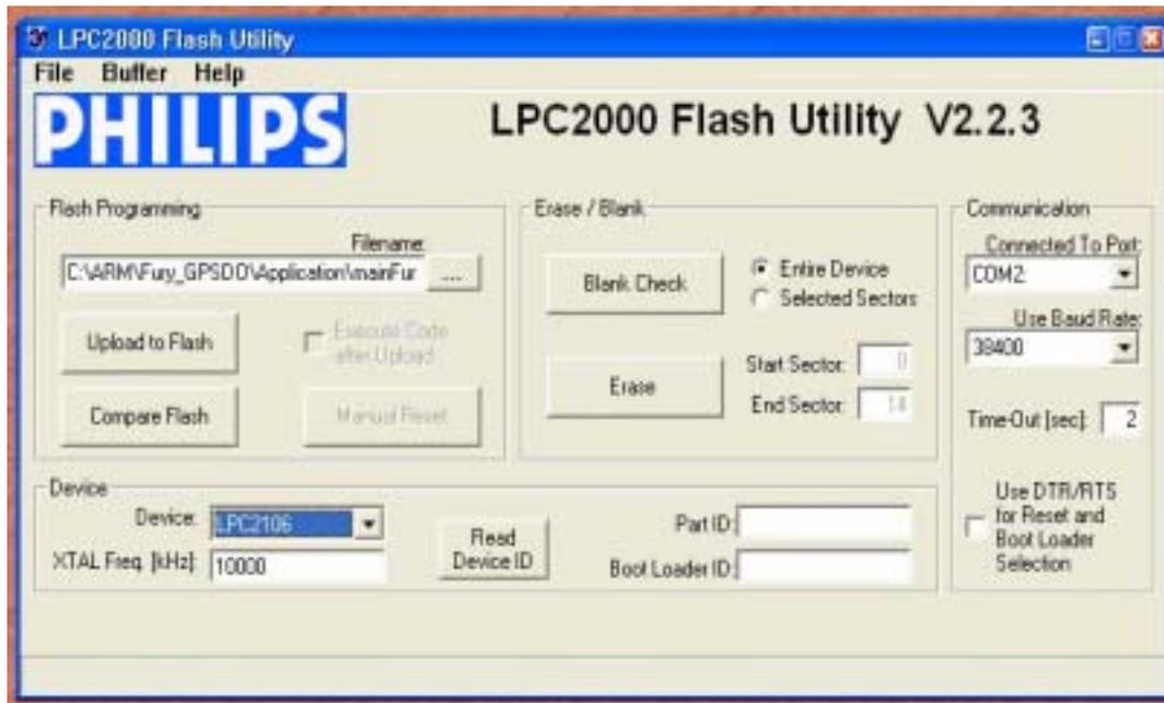
*Please note that the “Use Baud Rate” setting needs to be set to 38400 Baud or less, it will not work faster than 38400 Baud.*
