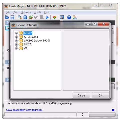
C) Expand the ARM7 folder and select the appropriate processor, in this case the LPC2138.
