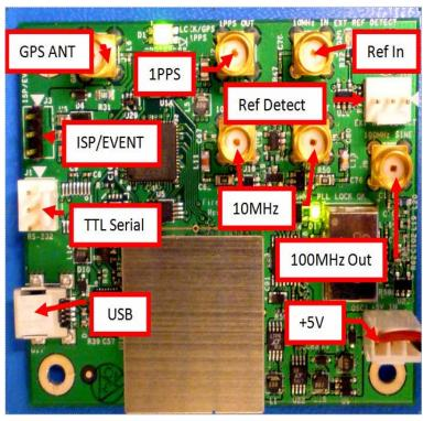
Figure 2.2 FireFly-1C PCB Mechanical Drawing
