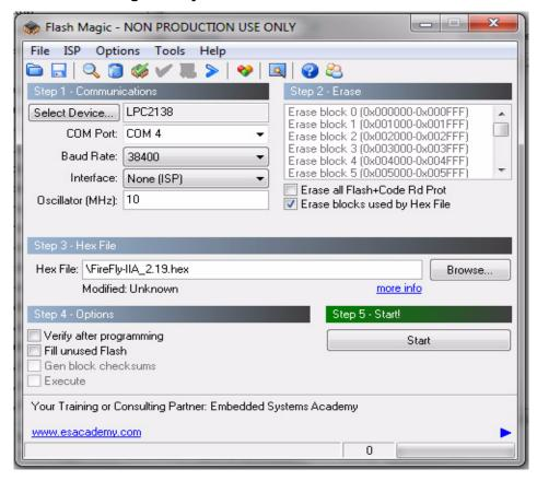
B) Press the "Select Device" button and the window shown in Figure 4.4 will appear:
