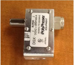
Polyphaser impulse suppressor. Included in kit PN:92-1330 only. Input is on the left and output is on the right. Grounding connection nut is connected on bottom.
